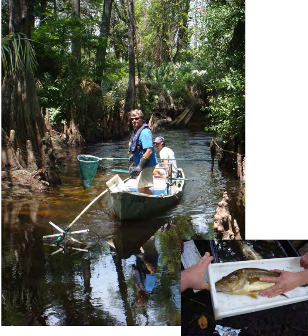
Figure 4-8. Motorized canoe equipped with generator and single anode for electroshocking in the Northwest Fork
