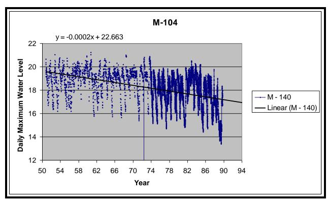
Figure 7 - Groundwater Levels in M-140
