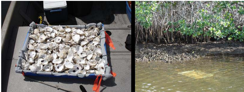
Figure 2: A benthic sampling tray filled with oyster shell (left) and a deployed tray (visible at low tide) located at one of the river's natural oyster reefs (right).
