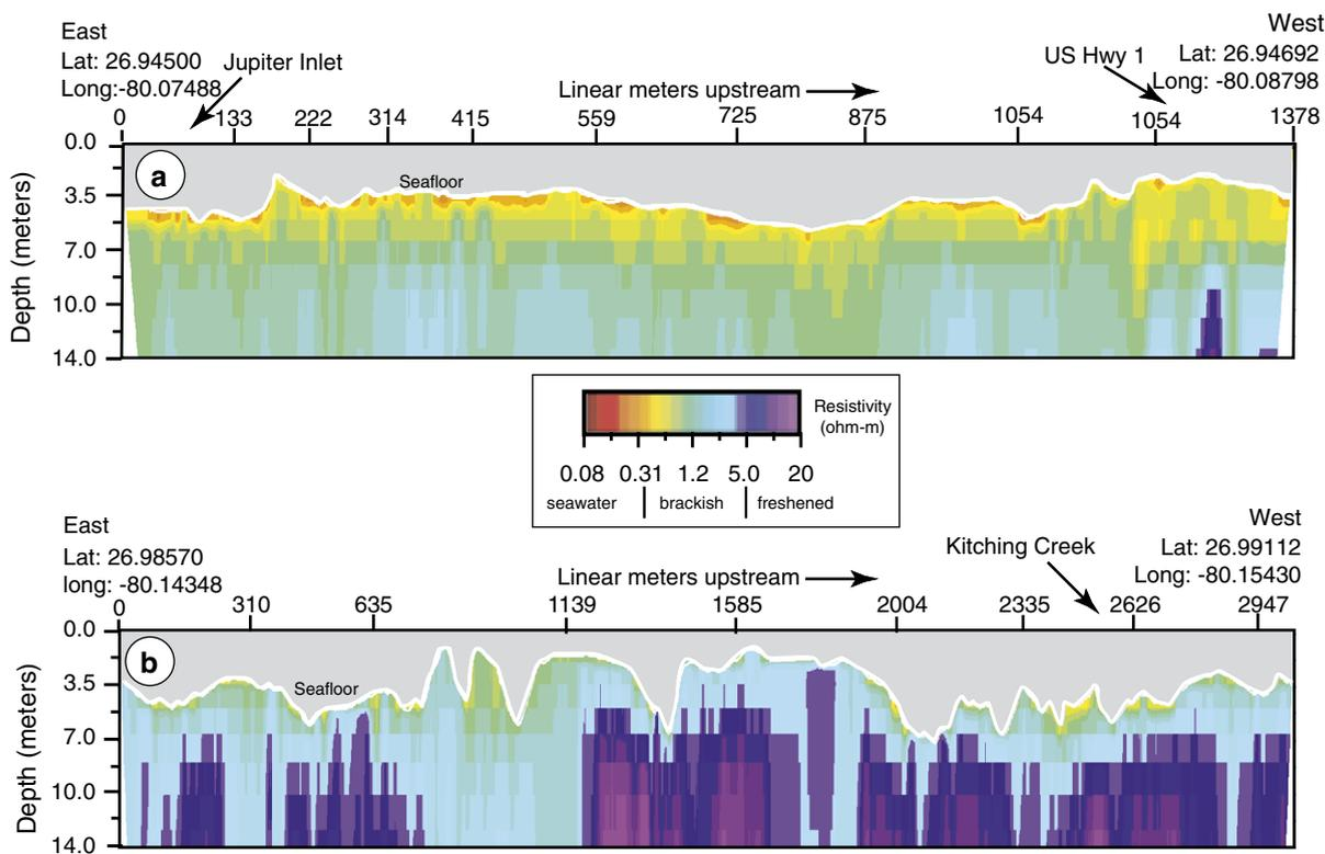
Fig. 7. A comparison of two modeled streaming resistivity profiles, (a) one proximal to Jupiter Inlet in a saline (salinity  $\sim 33$ ) environment, and (2) one upstream (salinity  $\sim 0$ ), close to the confluence of Kitching Creek and the Loxahatchee River.
