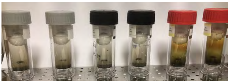
BART™ biological activity reaction test vials where microbes grow into formations of clouds, slimes and gels for different types of bacteria.
