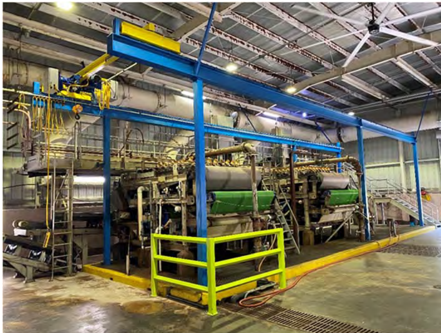
Sludge Dewatering Belt Filter Press Units and Bridge Crane
