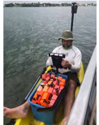
Staff using the new modular GPS system in the field. The great staff from our maintenance department fabricated mounting brackets for our kayak.
