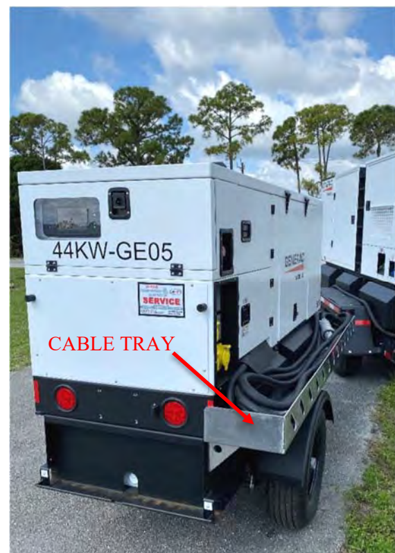
Towable Emergency/Standby Generator Unit – Cable Trays
