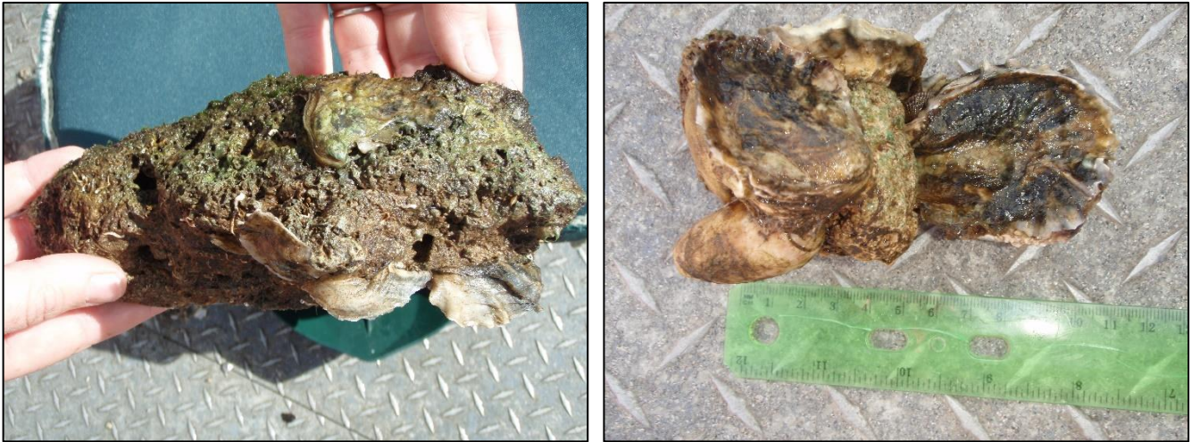
Photo 4. The NOAA restoration reefs were created using sandstone rock and various seashells that were undesired components of a local beach renourishment project. Photos show oysters attached to different size pieces of sandstone rock which appeared to exhibit the best results for recruiting oysters.
