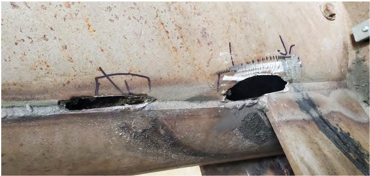
Grit Classifier Housing Failures
