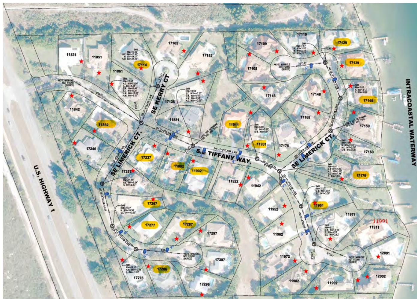
Figure 2. Existing Sanitary Sewer Laterals and Septic Tank Locations
