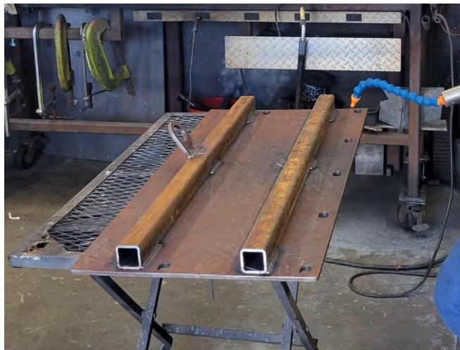
Temporary Weir Plate Fabricated by Maintenance Team
