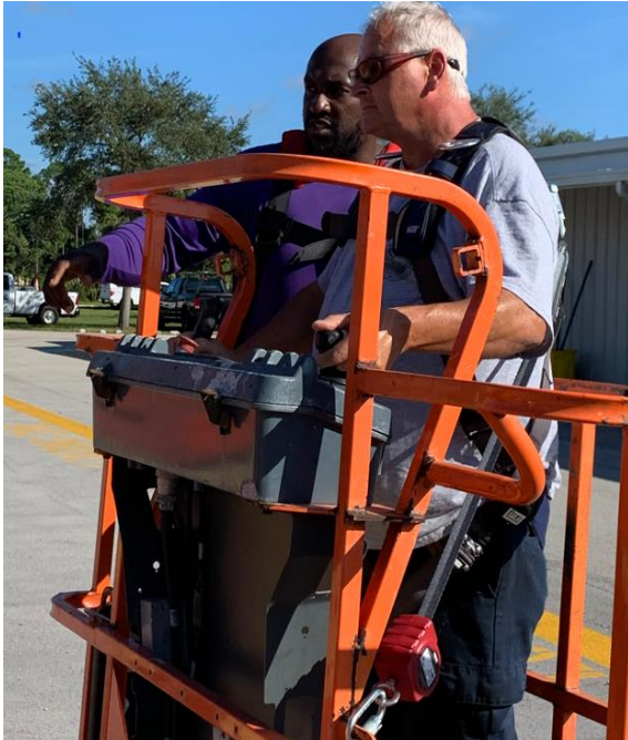
At left: Brian Davis and Chris Whalen testing the articulating boom controls during the practical certification. Both are using the required fall arrest harness and SRL lanyard. At right: Vince Beatrice and John Smith practicing safety at new heights during boom training certifications. Fall arrest training was provided to all users prior to the certification.
