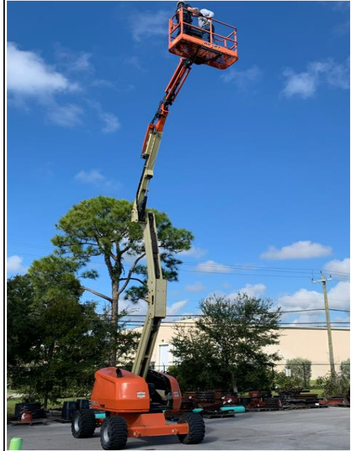
At left: Brian Davis and Chris Whalen testing the articulating boom controls during the practical certification. Both are using the required fall arrest harness and SRL lanyard. At right: Vince Beatrice and John Smith practicing safety at new heights during boom training certifications. Fall arrest training was provided to all users prior to the certification.
