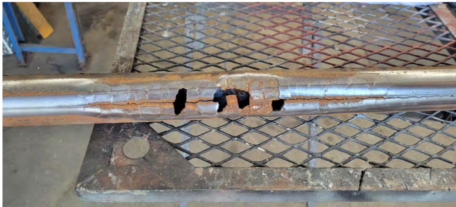
Site Access Gate No. 2 – Worn Section of Bottom Rail
