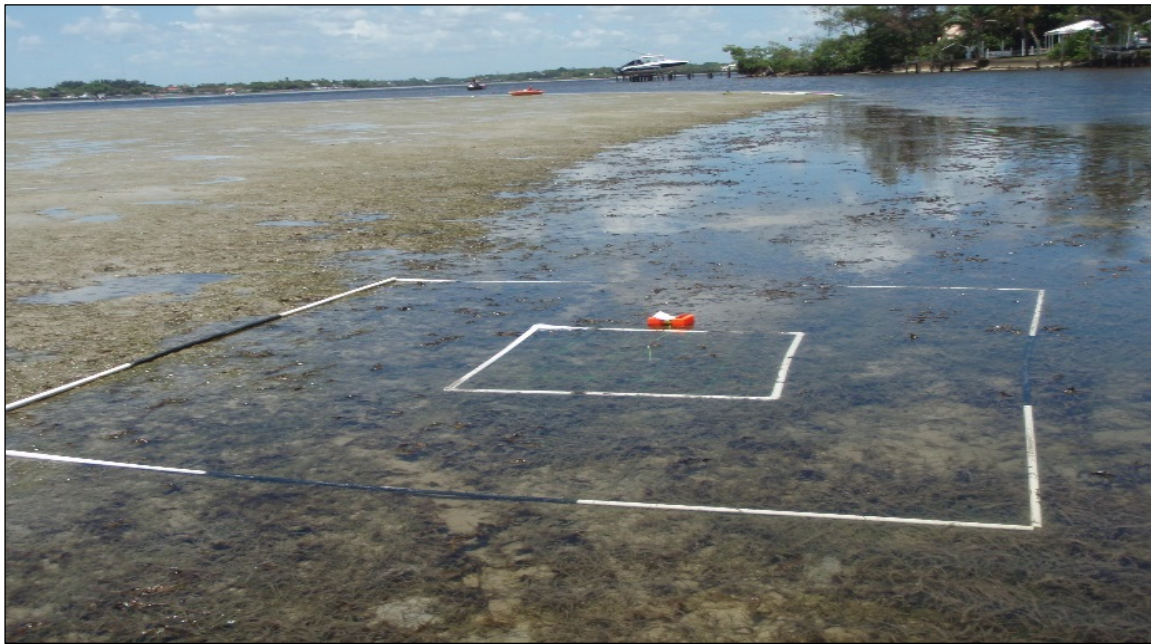
Figure 3. A 9m 2 collapsible sampling quadrat, centered on weighted marker buoy, at low tide. The smaller 1m 2 quadrat is shown for scale. Seagrass categories were based on the number of 1-meter squares within the quadrat occupied by seagrass and include Continuous (7-9), Patchy (4-6), Sparse (1-3), and Absent (0).
