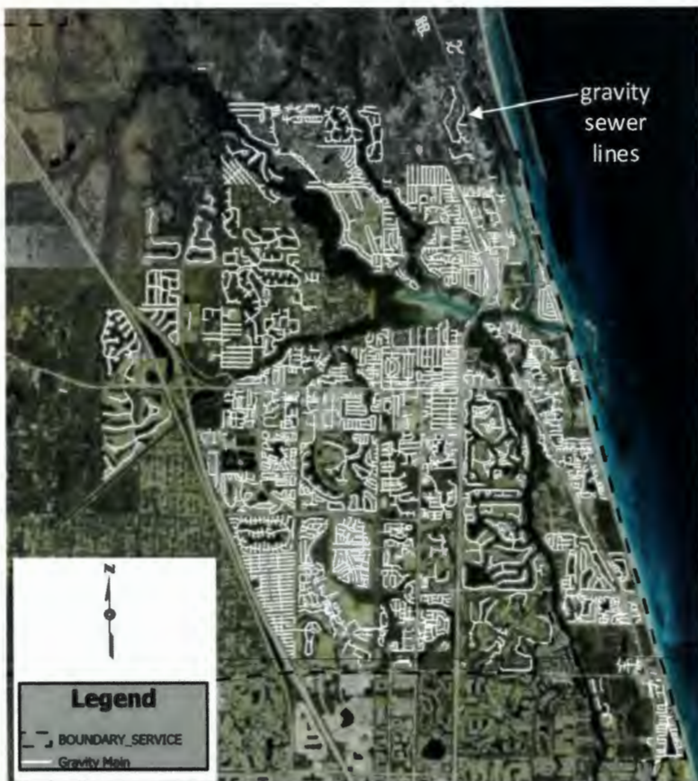
LRD Gravity Line System Overview
